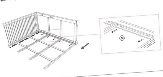
Tighten with bolts (N) with ALLEN KEY 6MM according to the code
